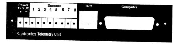
Power – The supplied power cable will plug into the rear panel terminal strip marked Power and connect to your 12 volt DC power supply.
