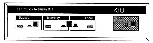
Bypass LED (Red) – When the BYPASS switch is depressed, this LED will light, indicating that the KTU is in the BYPASS mode, connecting your attached terminal to the TNC. The BYPASS switch must be in the OUT position for KTU operation to either the TNC or the terminal.
