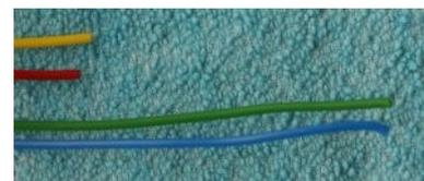
Leaving the green and blue wires 5cm longer than the red and yellow allows the cables to be neatly coiled once fitted to the board, as the longer pair go to the opposite side of the board.
