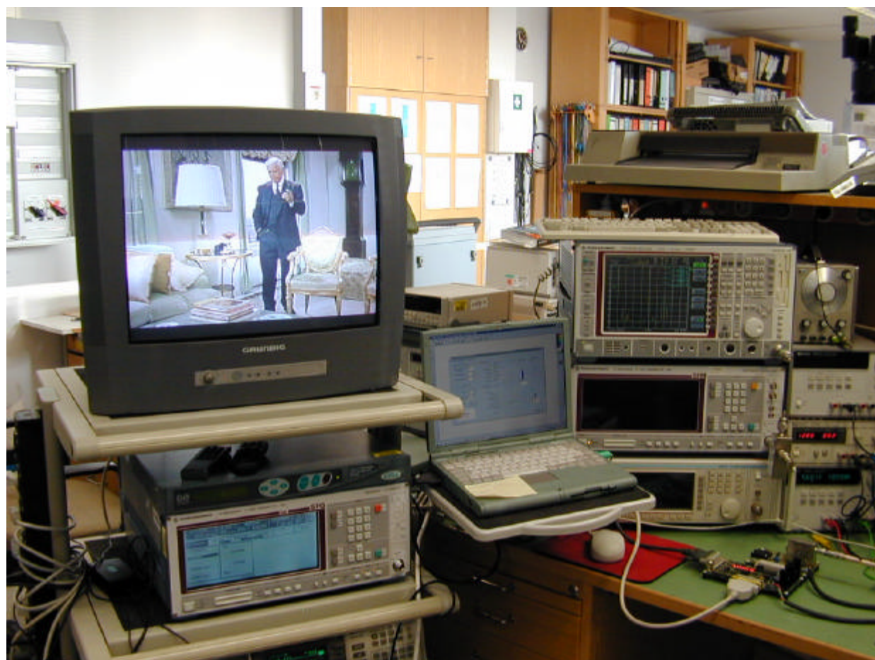
Fig.3 DVB-T Test Set-up and the Received Program
