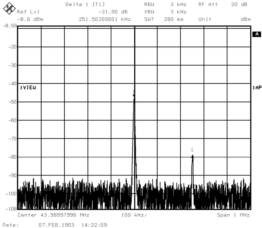
**Fig. 33 Tuner Output Signals, Internal AGC take-over point=106dBuV**
