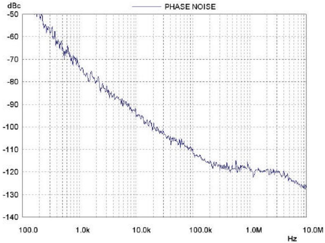
Fig. 9 VHFL, RF=159MHz,  $I_{cp}=50\mu A$ ,  $f_{ref}=62.5KHz$
