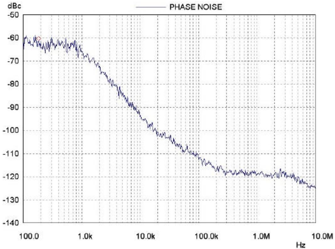
Fig. 20 UHF, RF=651MHz,  $I_{cp}=125\mu A$ ,  $f_{ref}=62.5KHz$
