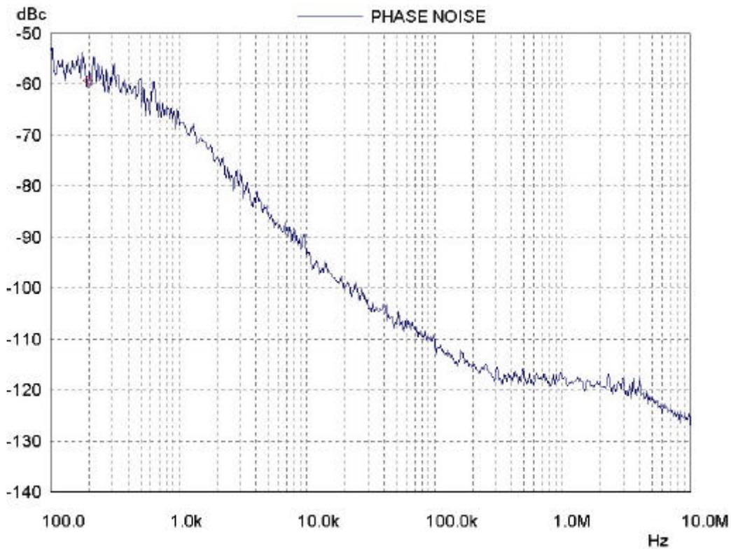
**Fig. 23 UHF, RF=861MHz,  $I_{cp}=650\mu A$ ,  $f_{ref}=62.5KHz$**
