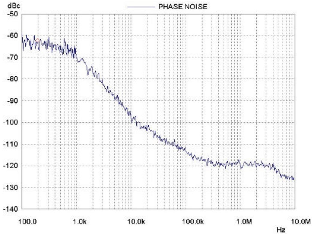
Fig. 13 VHFH, RF=303MHz, **Icp=50uA**, fref=62.5KHz
