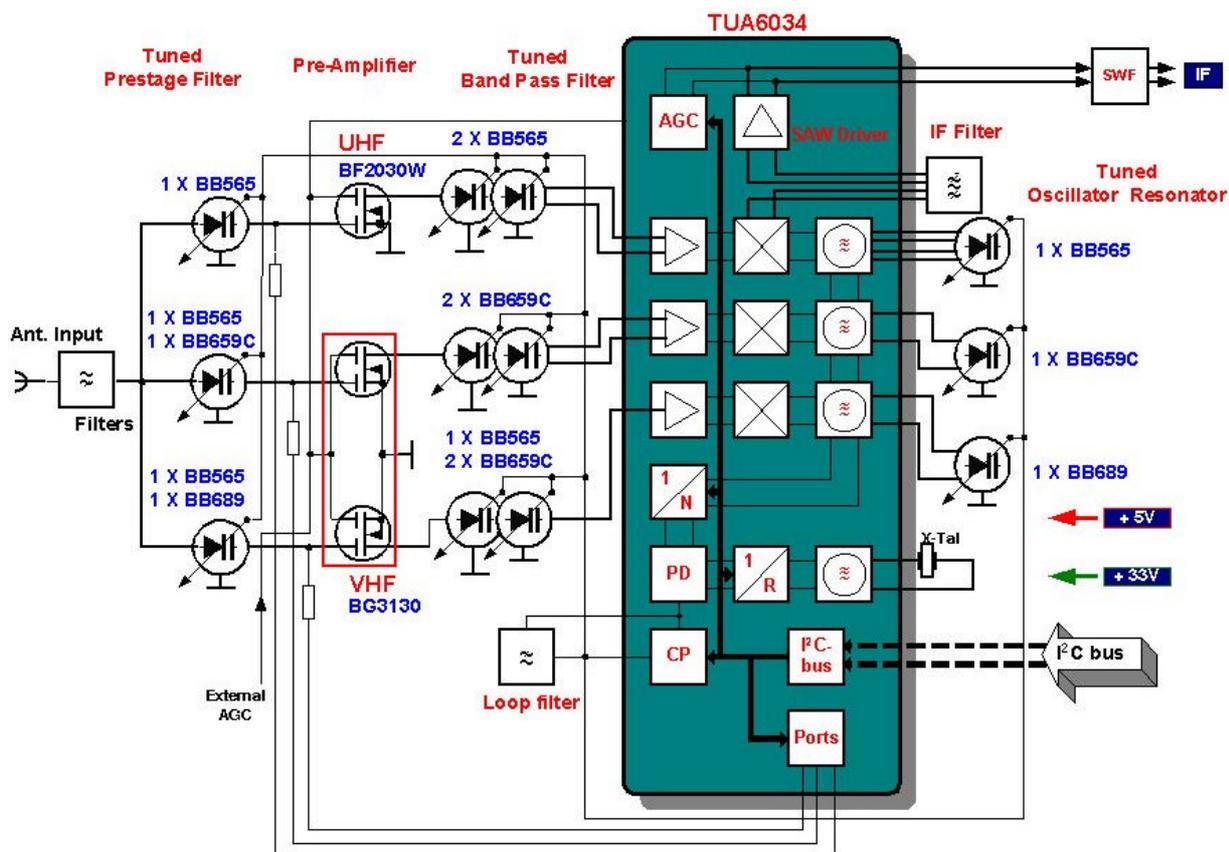
Fig. 4 Block Diagram of the ATSC Tuner with TUA6034
