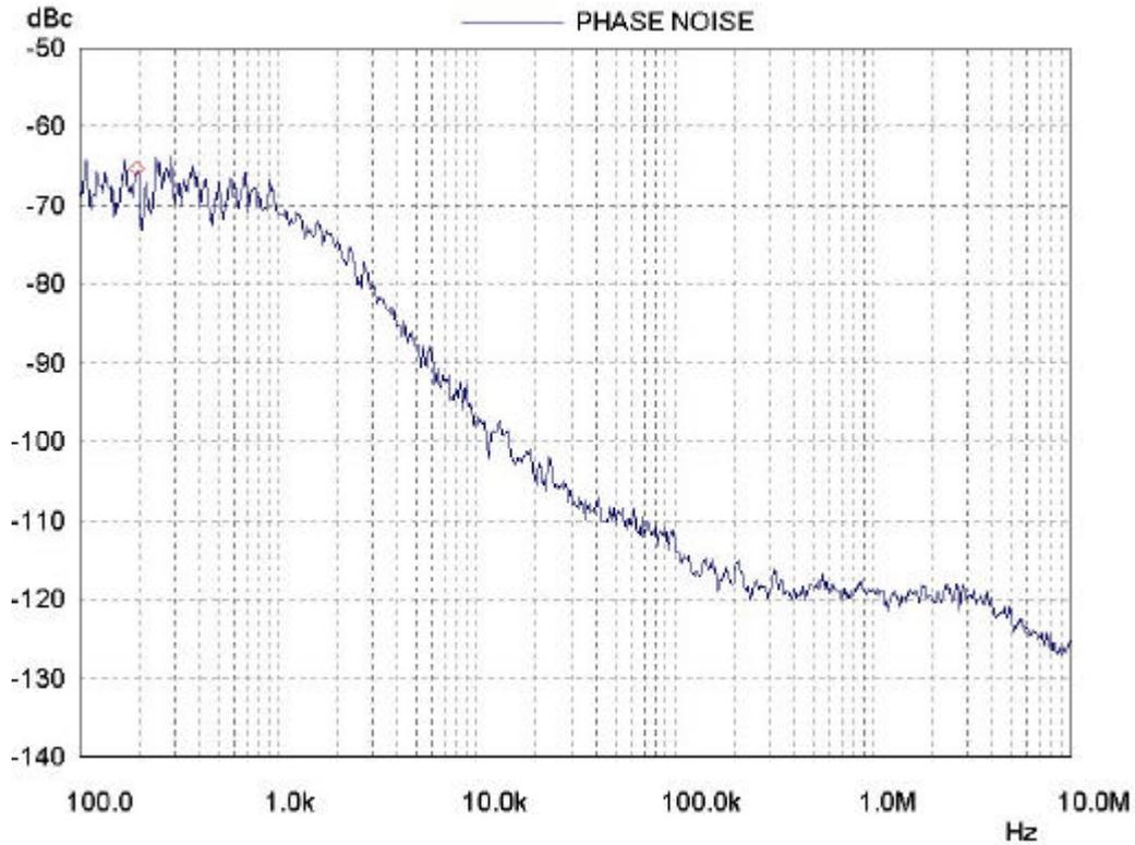
Fig. 14 VHFH, RF=303MHz, **Icp=125uA**, fref=62.5KHz
