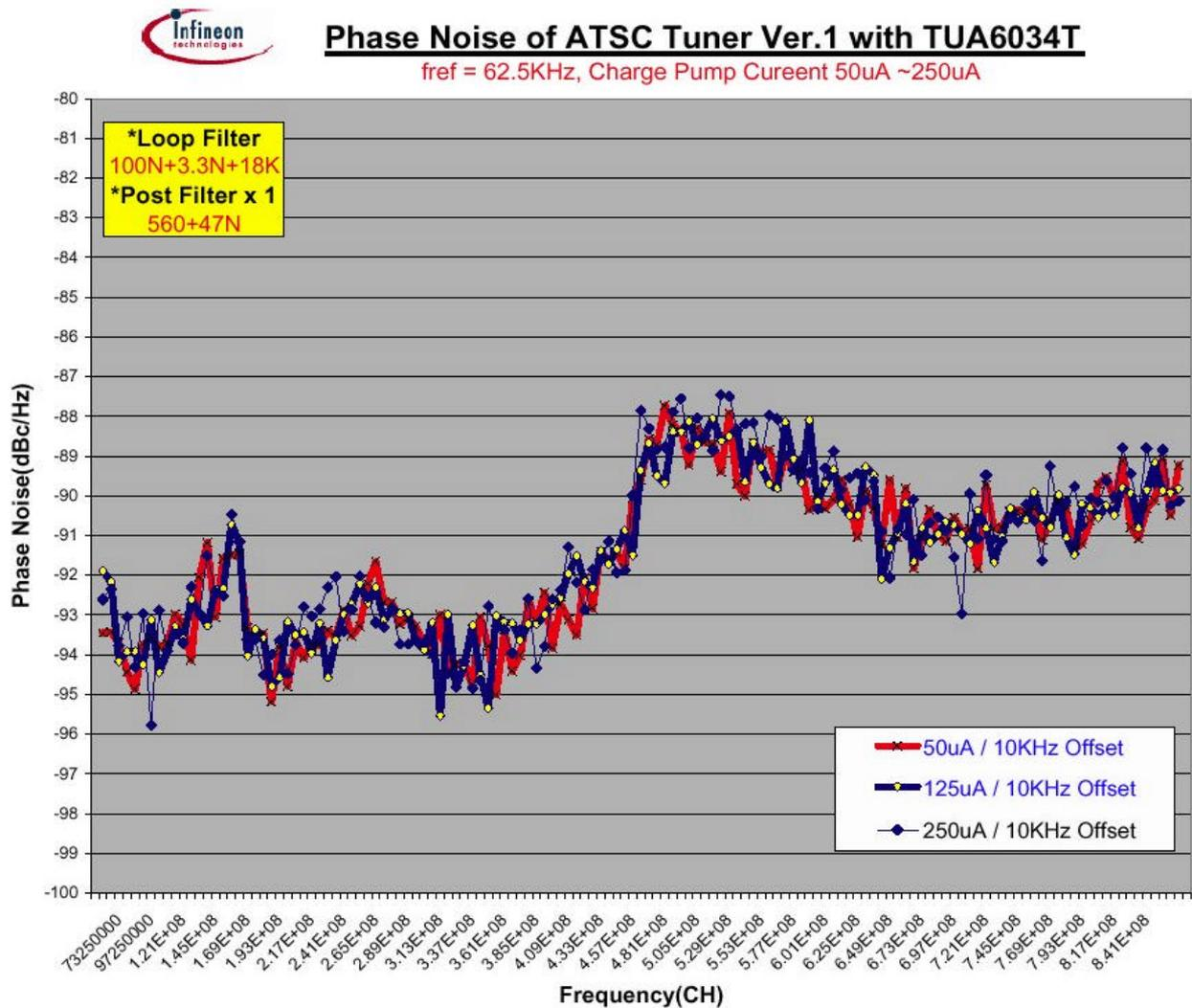
**Fig. 6 Phase Noise in the whole frequency range at 10KHz offset**
