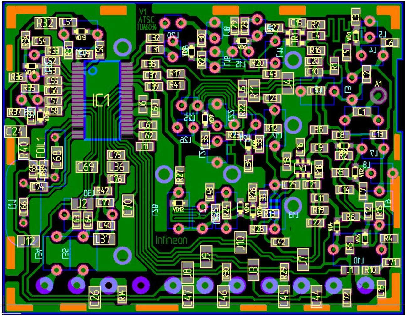
Fig. 5 PCB Layout of the ATSC Reference Tuner with TUA6034-T
