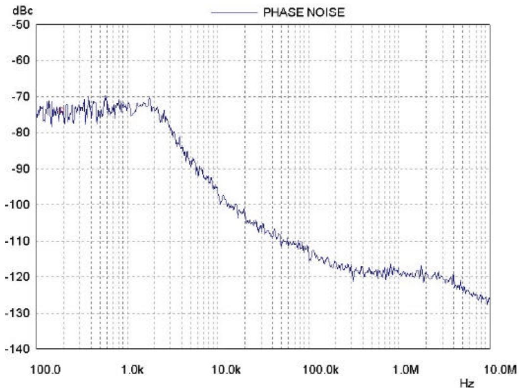
Fig. 12 VHFH, RF=165MHz, **Icp=125uA**, fref=62.5KHz
