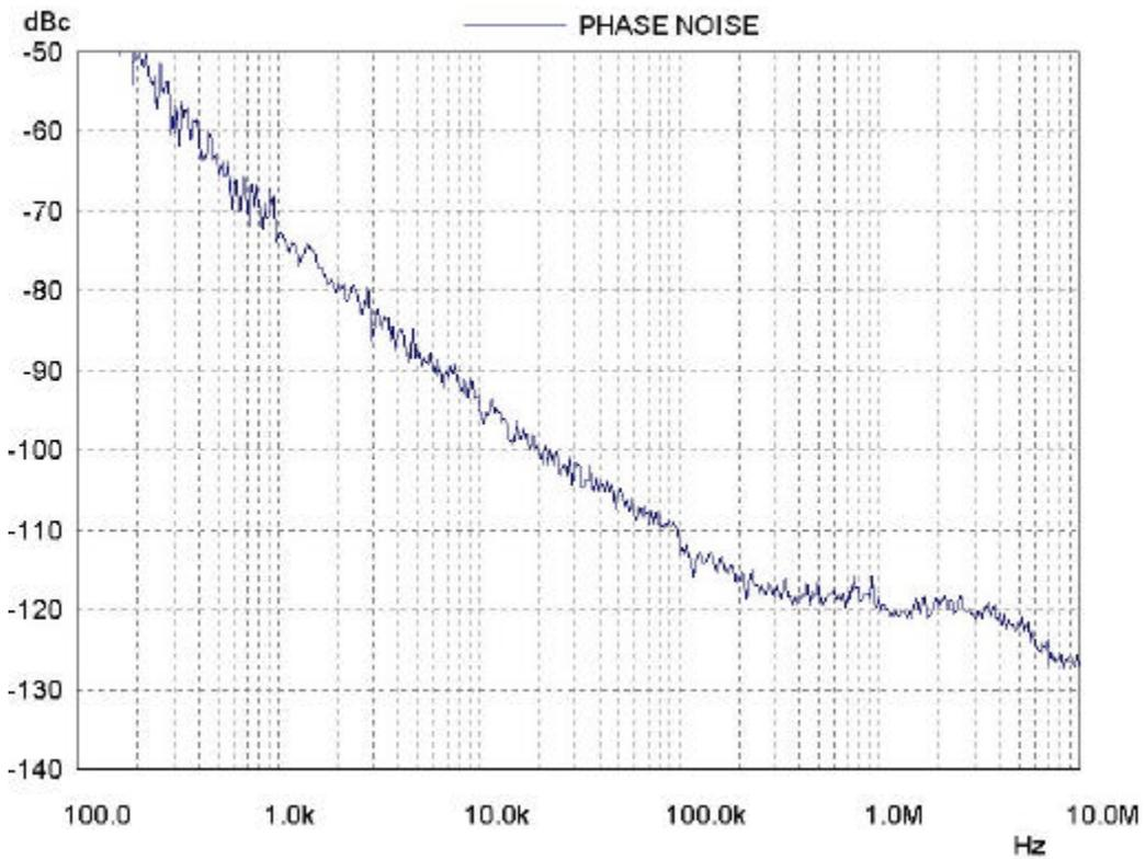
Fig. 10 VHFL, RF=159MHz,  $I_{cp}=125\mu A$ ,  $f_{ref}=62.5KHz$
