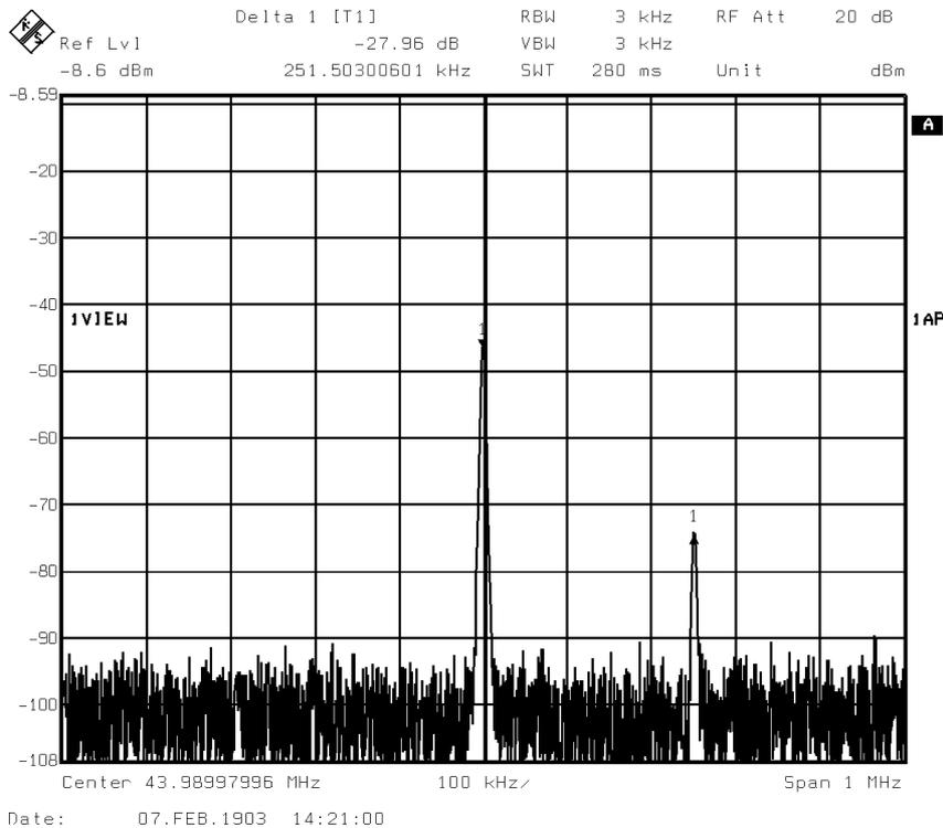
**Fig. 34 Tuner Output Signals, Internal AGC take-over point=109dBuV**
