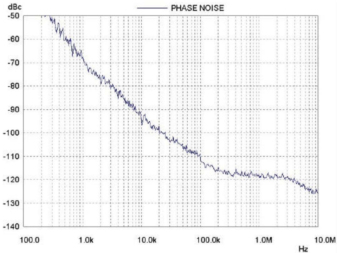
Fig. 22 UHF, RF=861MHz,  $I_{cp}=125\mu A$ ,  $f_{ref}=62.5KHz$
