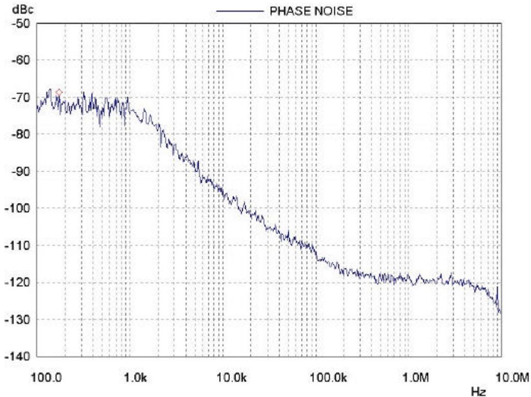
Fig. 8 VHFL, RF=57MHz,  $I_{cp}=125\mu A$ ,  $f_{ref}=62.5KHz$
