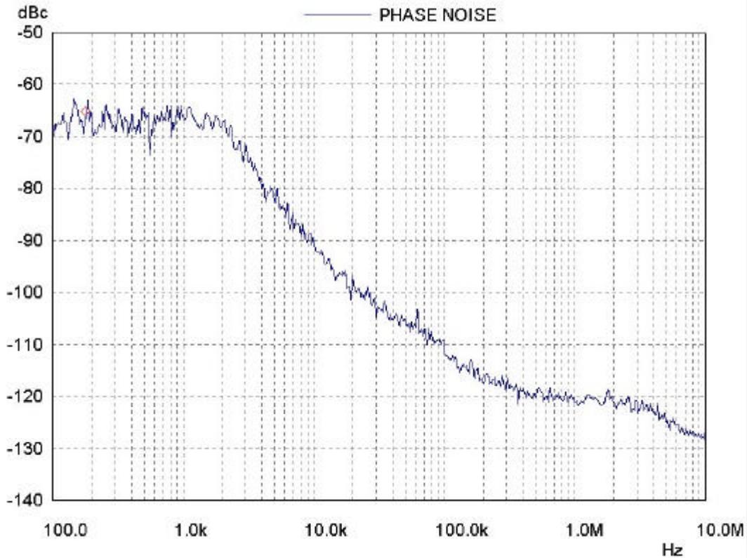
Fig. 18 UHF, RF=459MHz,  $I_{cp}=125\mu A$ ,  $f_{ref}=62.5KHz$
