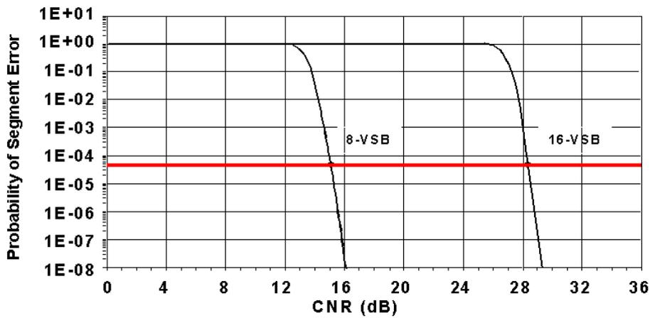
**Fig. 2 Probability of Segment Error for 8VSB-T and 16VSB<sup>2</sup>**
