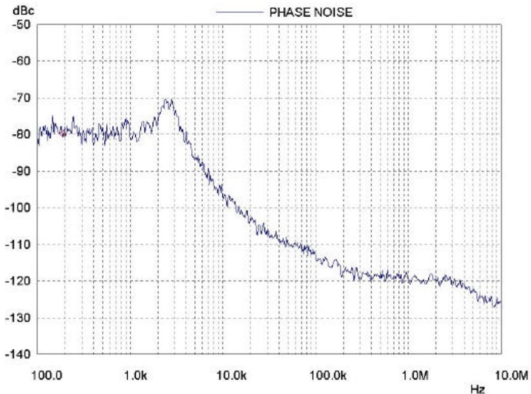
**Fig. 24 VHFH, RF=165MHz,  $I_{cp}=250\mu A$ ,  $f_{ref}=62.5KHz$**
