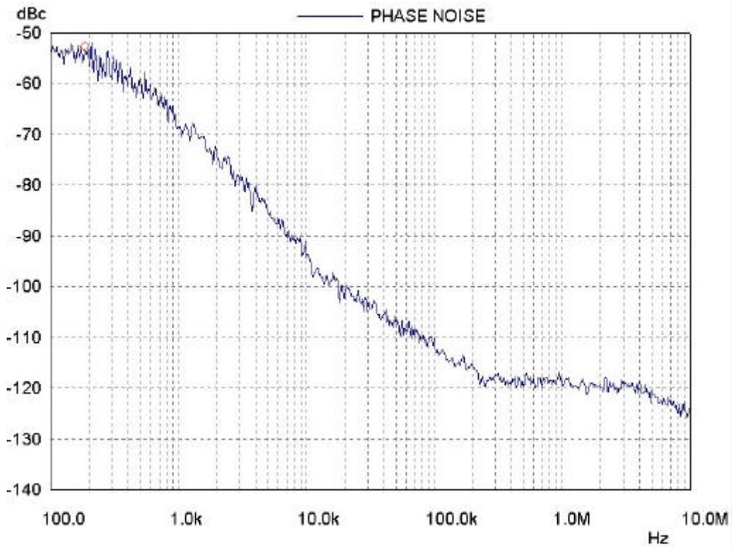
Fig. 19 UHF, RF=651MHz,  $I_{cp}=50\mu A$ ,  $f_{ref}=62.5KHz$
