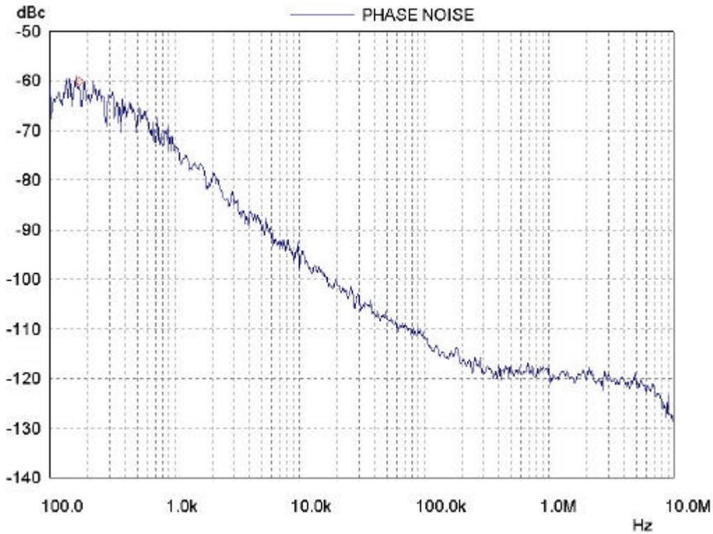
Fig. 7 VHFL, RF=57MHz,  $I_{cp}=50\mu A$ ,  $f_{ref}=62.5KHz$
