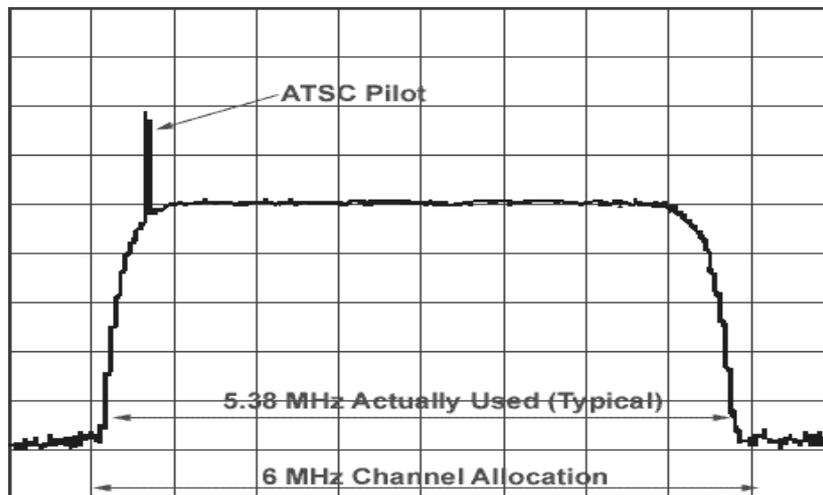
**Fig. 1 An example of a typical ATSC (8-VSB) signal**
