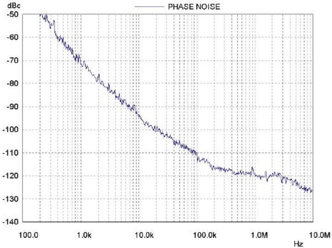
Fig. 15 VHFH, RF=453MHz, **Icp=50uA**, fref=62.5KHz
