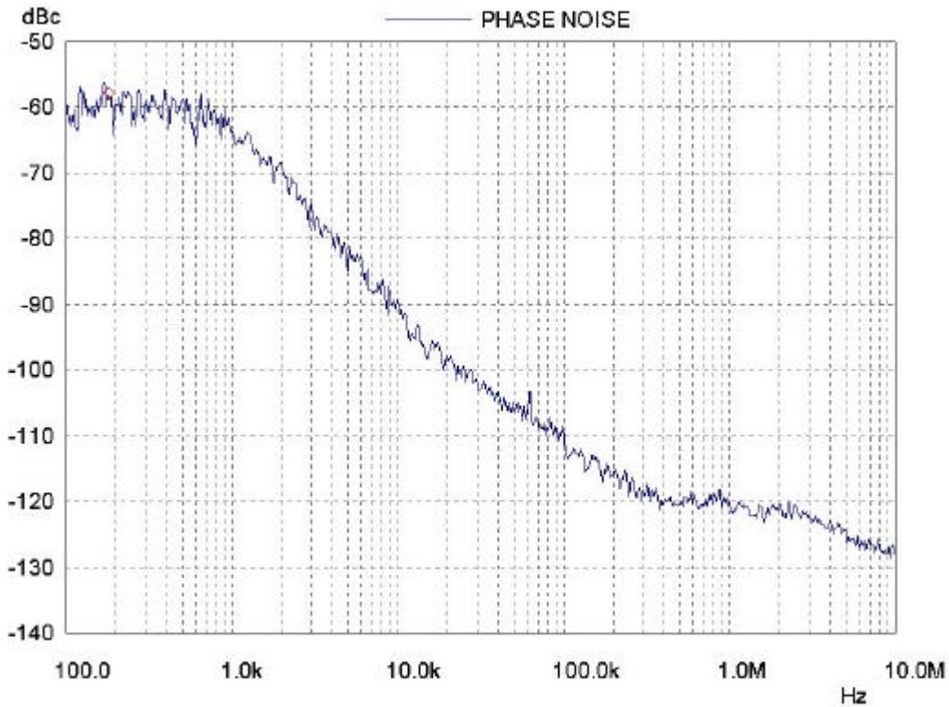
Fig. 17 UHF, RF=459MHz,  $I_{cp}=50\mu A$ ,  $f_{ref}=62.5KHz$
