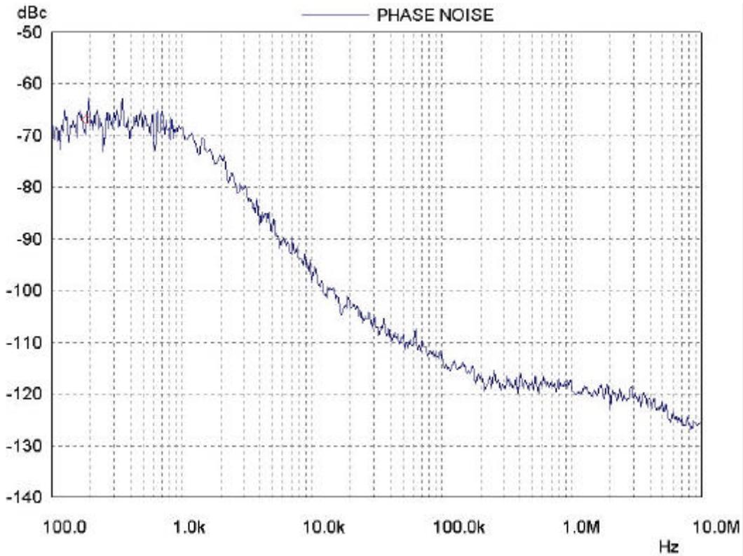
Fig. 11 VHFH, RF=165MHz, **Icp=50uA**, fref=62.5KHz
