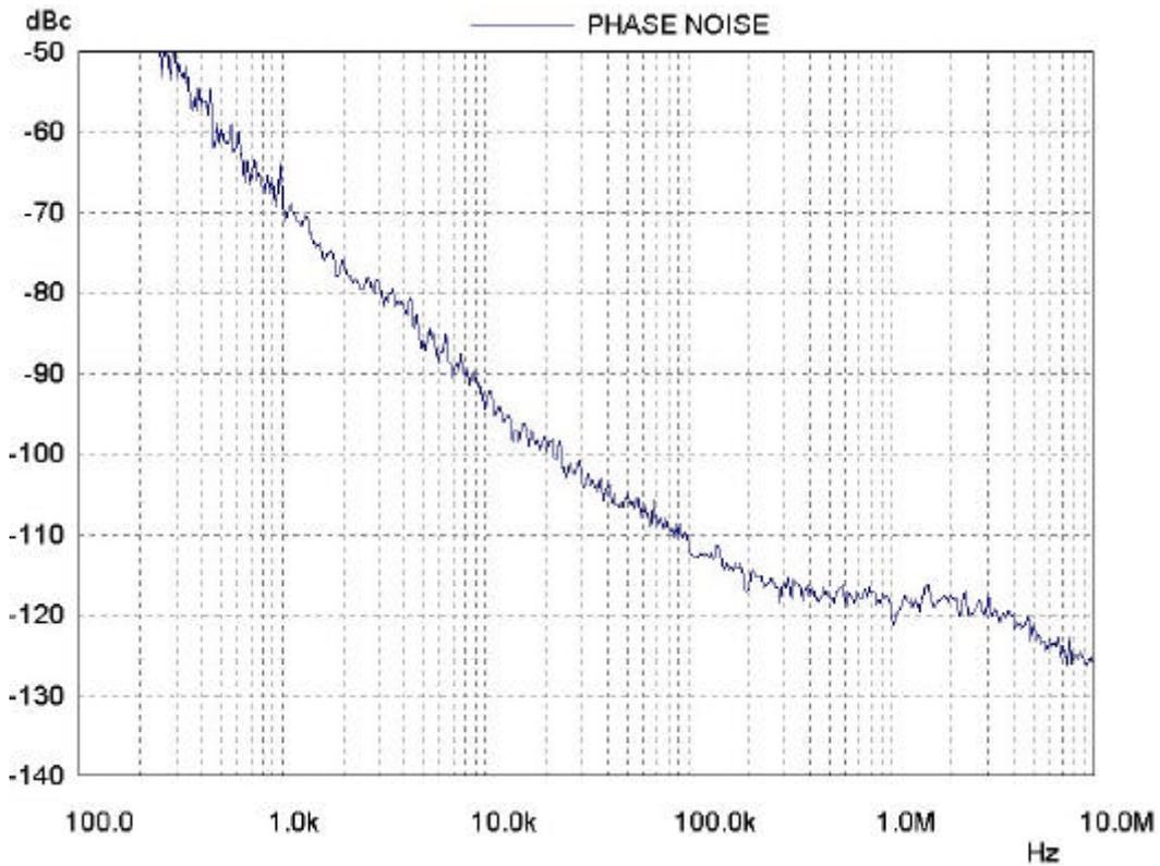
Fig. 21 UHF, RF=861MHz,  $I_{cp}=50\mu A$ ,  $f_{ref}=62.5KHz$
