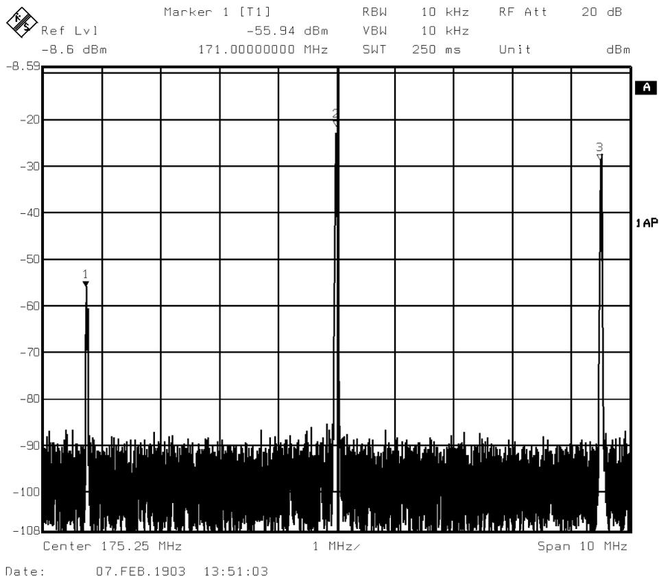
**Fig. 31 Tuner Input Signals for Intermodulation test;**
